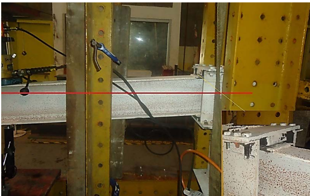
Figure 10. Damage state of the isolated connection
