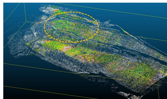
Figure 23. The surface deviation analysis with the output from the Iterative Closest Point (ICP) method From Figure 23, it can be seen that mobile laser scanner data can be used to map the changes between two epoch observations. The area marked with a dotted line indicates the
