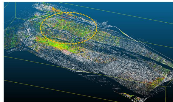
Figure 26. The surface deviation analysis with the output from the Align Point Pairs Picking registration method
