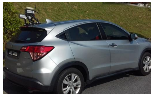
Figure 8. Data collection with mobile laser scanning equipment
