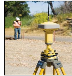
Figure 3. CPs Establishment through GPS observation
