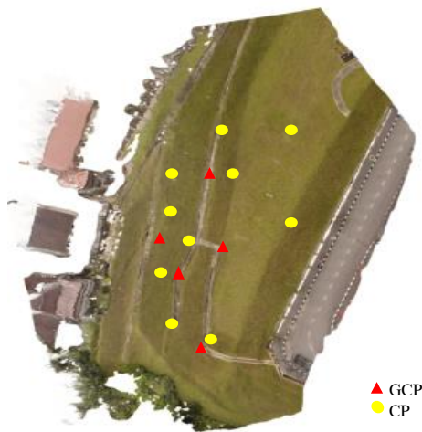
Figure 5. Distribution of GCPs and CPs of the slope area
