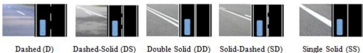
Figure 1. Road markers found at two-way non-urban road
