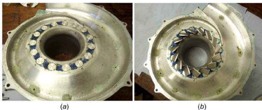
Fig. 4 Experimental setup that shows (a) vaneless turbine and (b) vaned turbine
