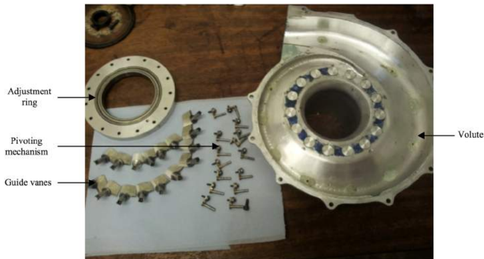
Fig. 3 Components of the turbine stage that include the volute, pivoting mechanism, lean vanes and adjustment ring
