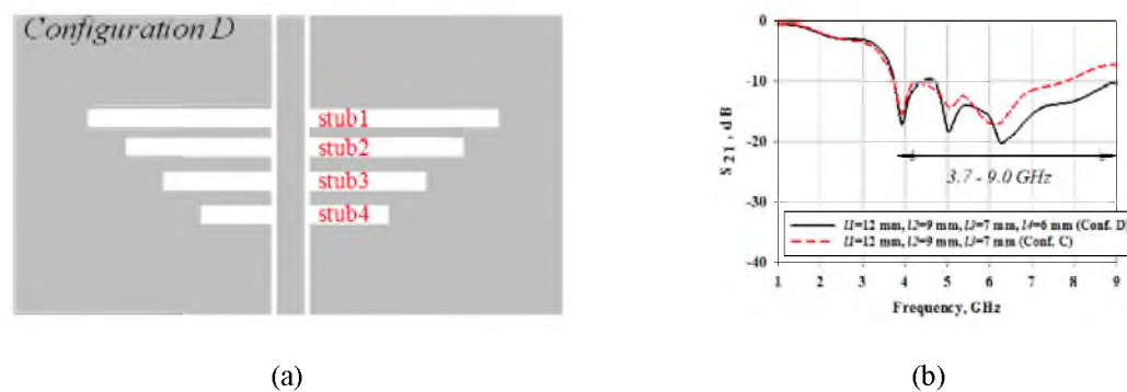
Figure 5. (a) Configuration D - quad-lines, rectangle slot (b) S_{21} result; configuration D vs configuration C
