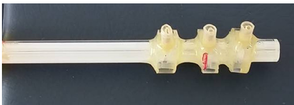
Fig. 12. Picture of pressure tap holder.
