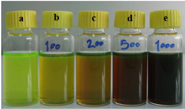
Fig. 8. Samples of CRC-CQDs after 6 months, (a) base fluid and (b–e) nanofluids by different concentrations of 100–1000 ppm.
