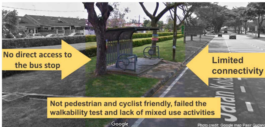
Figure 1.2 Design of transit station/stop that does not integrate with the surrounding area and responsive to the pedestrian accessibility
