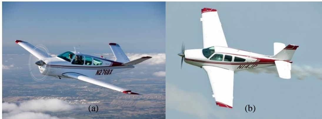
Figure 1.3 (a) V-tail Beechcraft Bonanza V35 (Flight Training Blog, 2012) and (b) Bonanza Conventional Aircraft (Aircraft in Focus, 2016)
