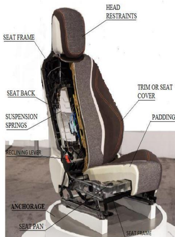
Figure 1 - Cut Section of Driver Seat Components and Systems 2
