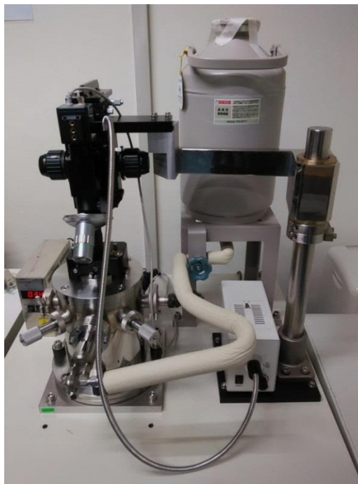
Figure A.6 : Atomic Force Microscope at Department of Physics, Faculty of Science, UTM.
