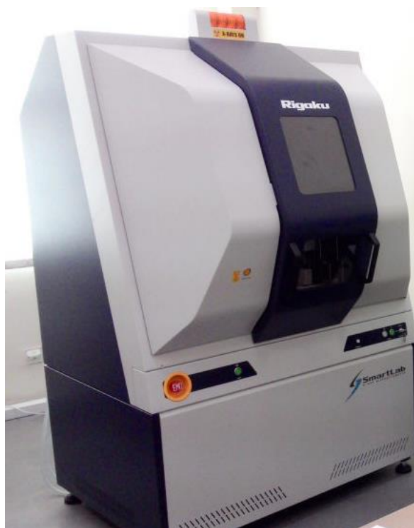
Figure A.2 : Rigaku SmartLab X-ray diffractometer available at University Industry Research Laboratory, UTM.
