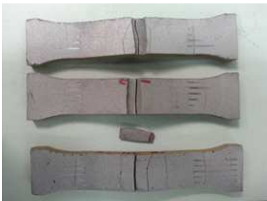
Fig. 9 Visible cracks after compression tests
