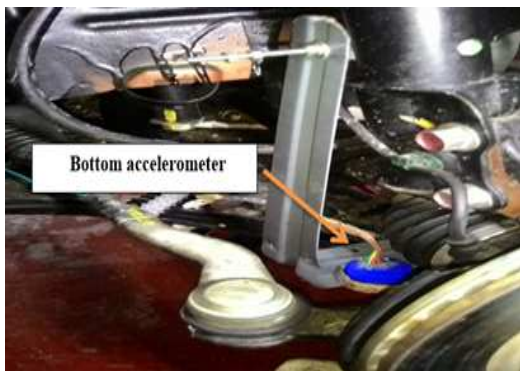
Fig. 4 Accelerometer sensor installation for vertical shaft acceleration
