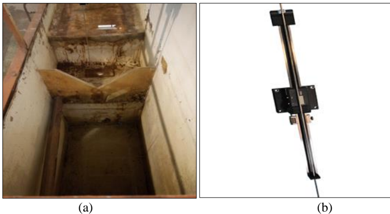
Figure 5: Flow measurement (a) a V-notch at the outlet, and (b) a point gauge to record water levels.
