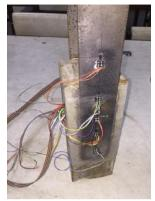
Figure 13: Sample SPECS-7 after installation of strain gauges
