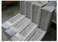
Figure 4: Readily hacked concrete surface
