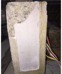
Figure 28: Concrete from SPECS-7 after failure
