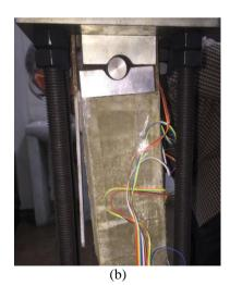
Figure 26: Debonding on one side of the concrete prism of SPECS-7
