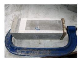
Figure 1: Concrete prisms attached with G-clamp prepared in 2008
