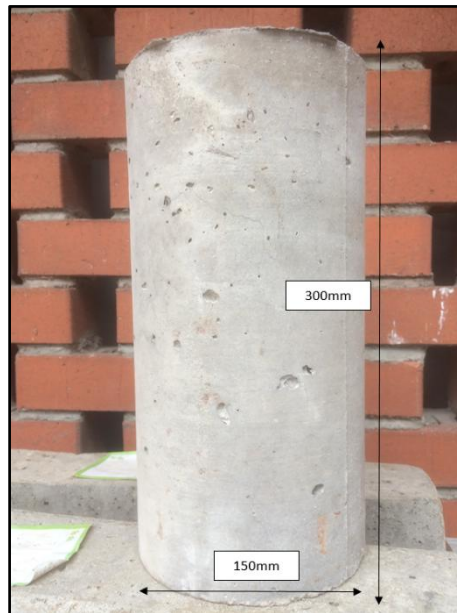
Figure 1: Cylinder specimens used in this study
