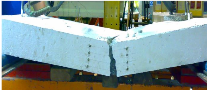
Figure 9: Failure mode of plain concrete slab (SC-PLAIN)
