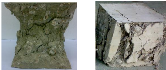
Figure 3: Failure of control concrete (left) and steel fibre concrete (right)
