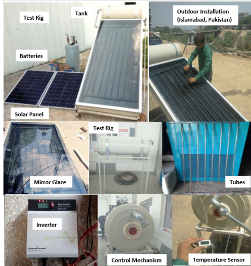
Figure 1 – Experimental setup; (a) Over all test rig, (b) Installation, (c) Mirror glaze, (d) Analytical model, (e) Tubes, (f) Inverter and hybrid system, (g) Control mechanism, (h) Temperature sensor
