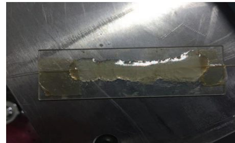
FIGURE 2: The c-PBT polymer after the heating process.
