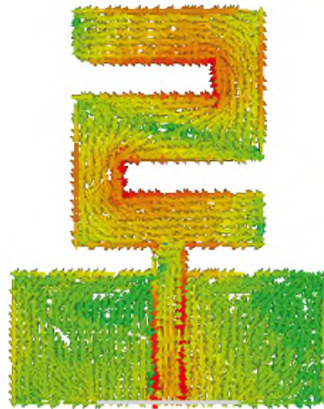
FIGURE 8: Simulated current distribution of the antenna at 2.45 GHz.
