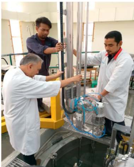
Fig. 9. Rig is carefully aligned before lowering it into the pool.
