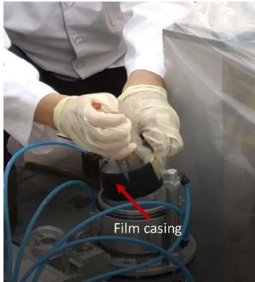
Fig. 15. Film is inserted into the compartment.
