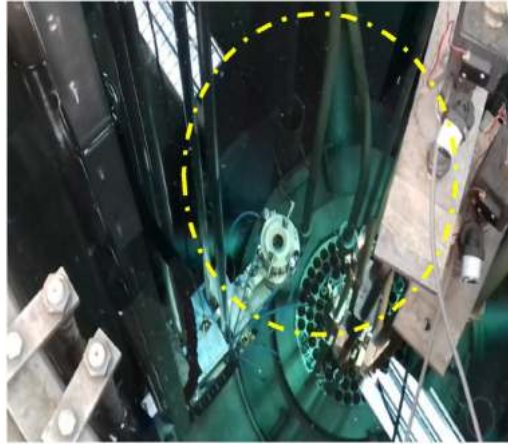
Fig. 11. Position of the underwater scanner in the pool (in circle).
