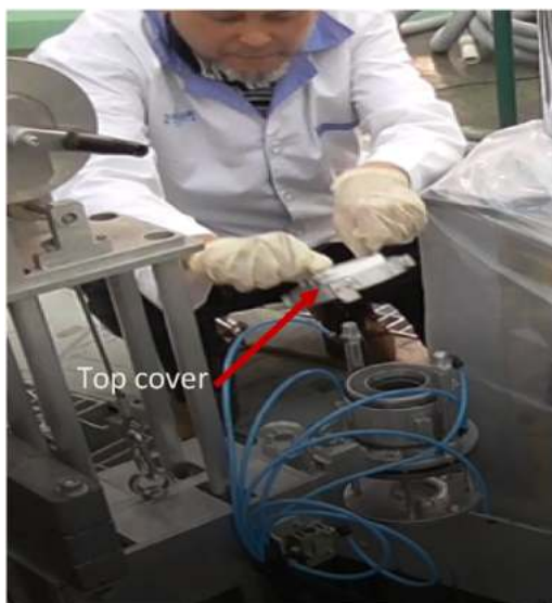
Fig. 13. Collimator cap is unscrewed and removed.
