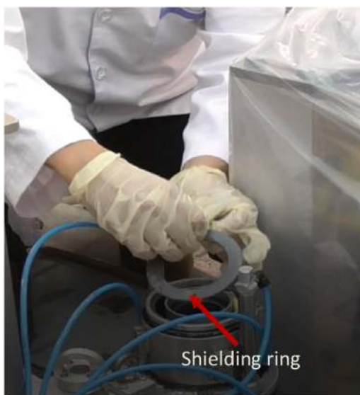
Fig. 14. The shielding ring is removed to get access to the film compartment.
