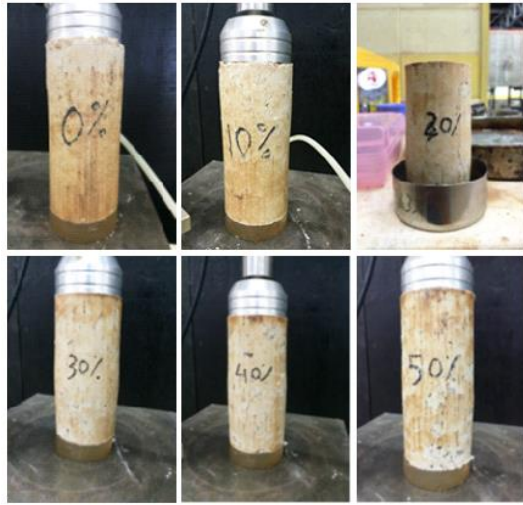
Fig. 11 Failure modes samples in UCS tests
