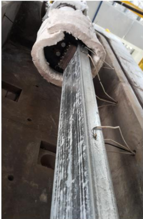
Fig. 3. Attachment of the thermocouple on the column.
