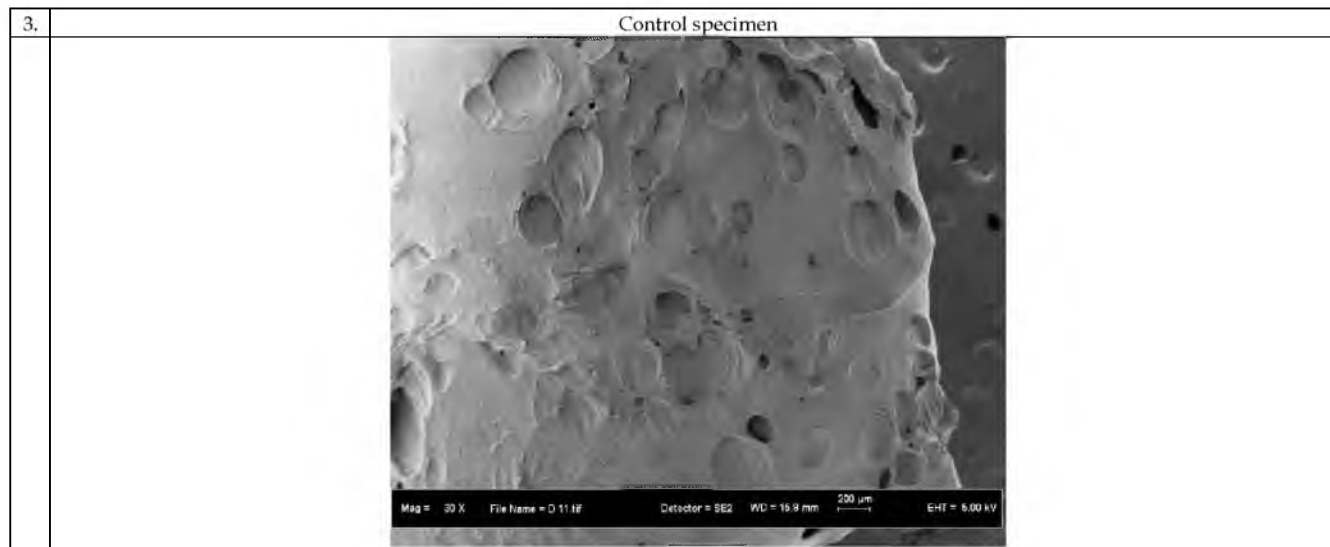
Figure 11. Cell morphology on the cross section of the 3D scaffolds after 7 days' cell seeding.
