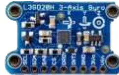
Figure 6. A 3-axis gyro sensor (Source: Adafruit Industries, 2017)
