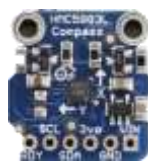
Figure 7. A 3-Axis magnetometer sensor (source: adafruit industries, 2017)
