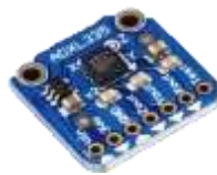
Figure 3. A 3-Axis accelerometer sensor (source: Adafruit Industries, 2017)
