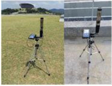
Figure 4 The probe is set up 300 mm above the ground to collect data
