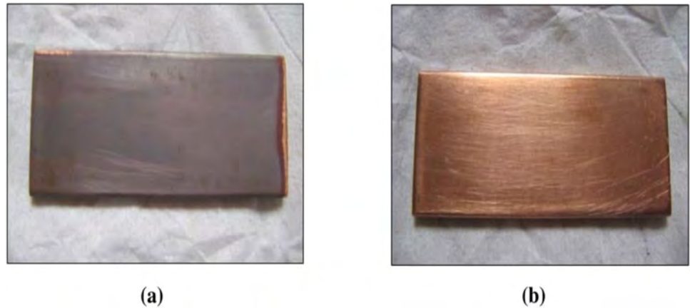
Fig 6. Copper specimen surface after corrosion test for 2 weeks period. (a) Without Treated Tannin Presence (b) With Treated Tannin Presence.
