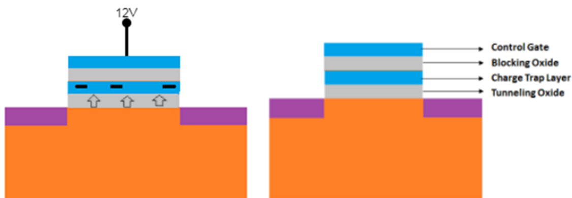
Figure 1.11: Charge trap Process and Labeling of Memory cell Layers
