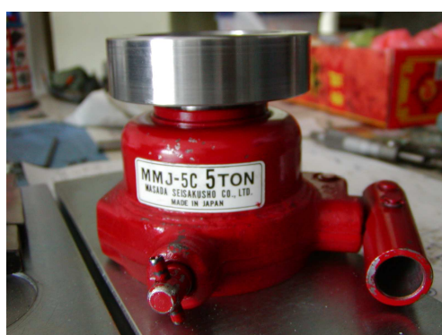
Figure 6: Mini hydraulic jack with capacity of 50 kN.
