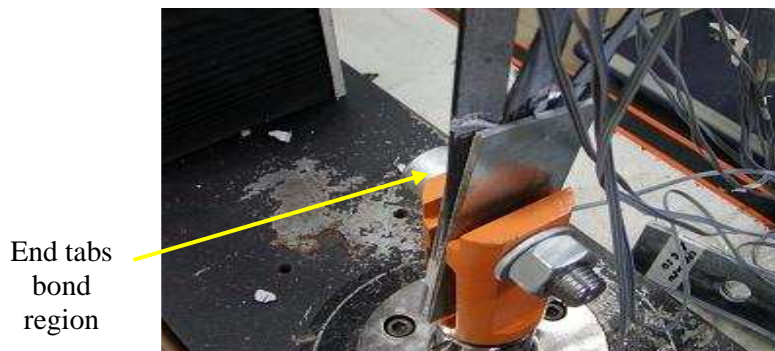
Figure 3: Close-up view of shear-out bond failure within mild steel end tabs CFRP plate under pull-pull load.
