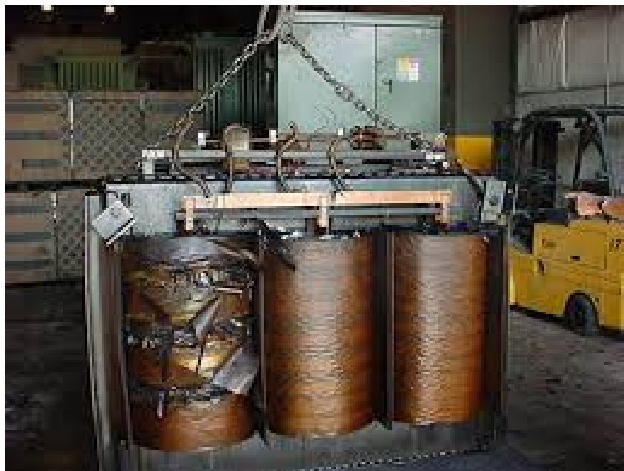
Figure 1.4: The Damage Of Winding Insulation
