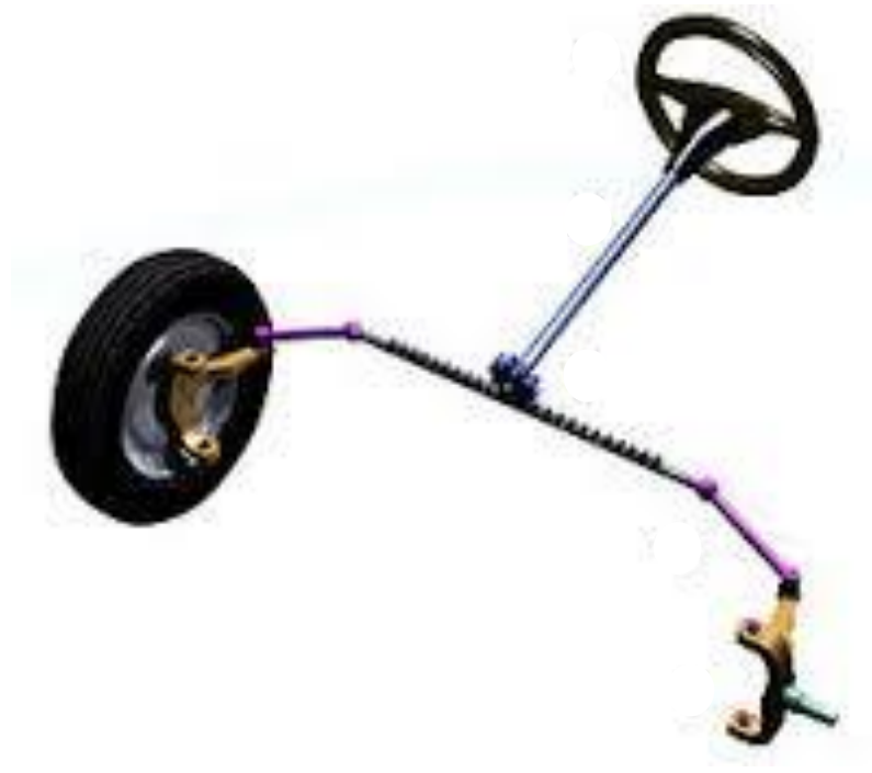
Figure 1.2 Rack and Pinion Steering System [2]
