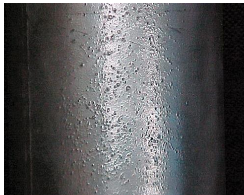
Figure 1.5: Pimples developed on galvanized steel surface due to dross interaction
