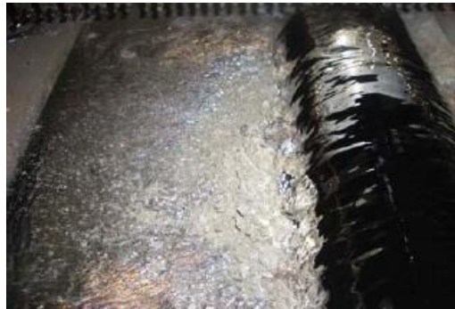
Figure 1.4: Dross formation covering surface of Zn-alloy molten bath
