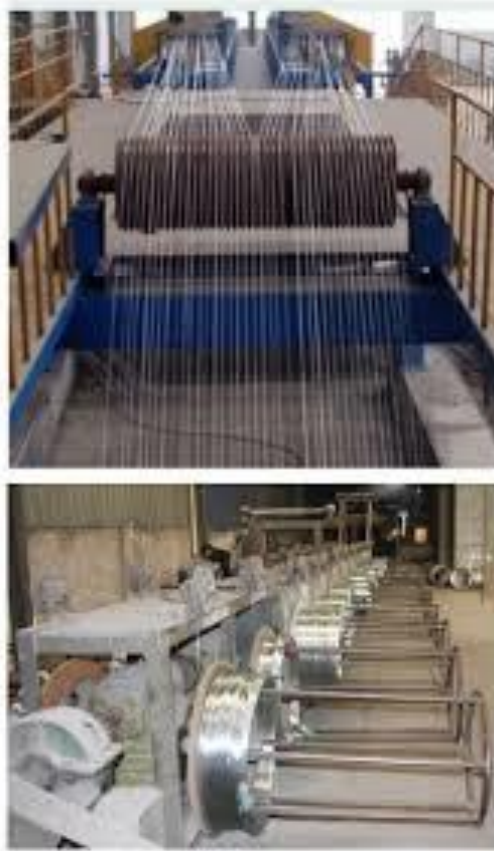
Figure 1.3: Steel wire rod ready to be hot-dipped in galvanizing bath
