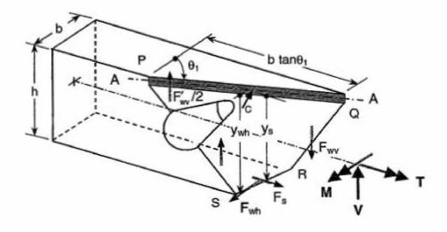
Figure 1.1Free Body Diagram of Beam with Opening under Torsion (Mansor1998)
