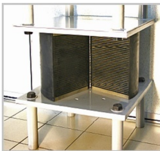
Figure 1.9 High damping rubber bearing (HDRB) showing internal layers
