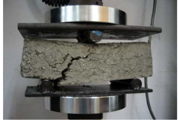
Figure 2. Three point flexural test.
