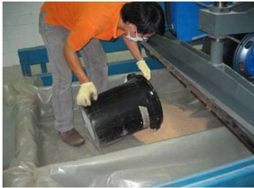
Figure 4: Screeding bedding sand
