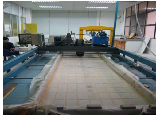
Figure 5: Concrete block tested pavement.
