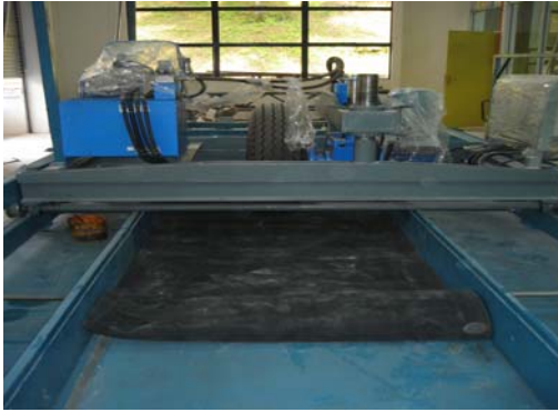
Figure 2: Hard neoprene on test bed
