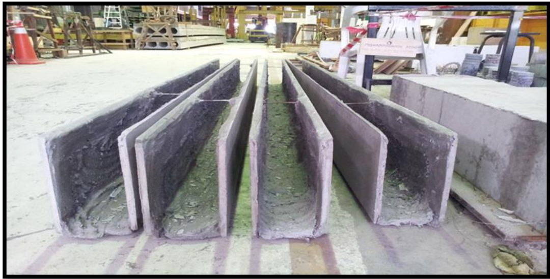
Figure 1.1 Sample of permanent precast formwork
