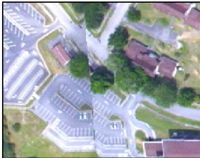
Figure 8 : Error that causes the road not connected perfectly
