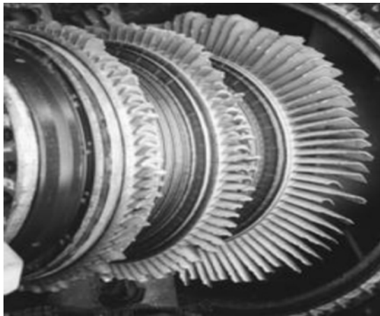
Catastrophic blades damage, source [10]
