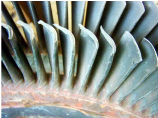
Deformation of rotor blades , Source: [8]
