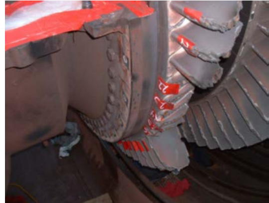
Failure of 1 st row of blades, Source [9]
