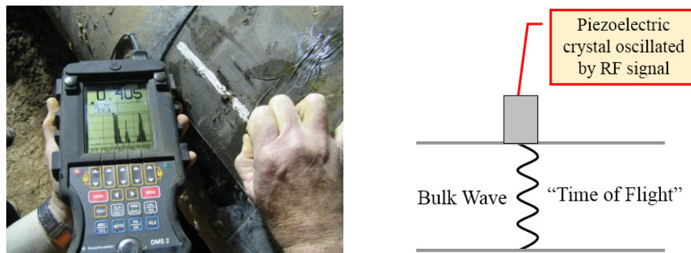
Figure 1.1 Principles of conventional UT
