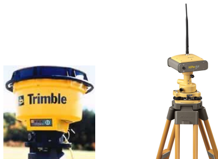
Figure 7: TRIMBLE 4800 GPS Receiver and Topcon HiPer GA Receiver
