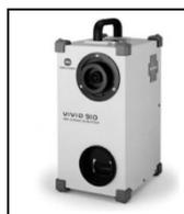
**Figure 2: Konica Minolta Vivid 910 laser scanner**
