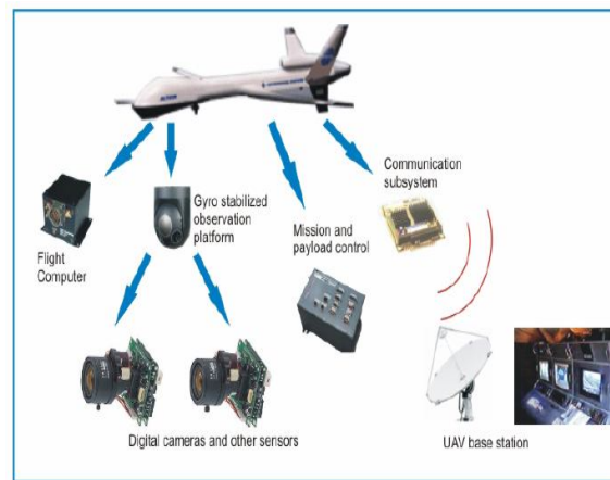
Figure 1: Main components of a UAV system.
