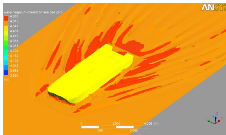
Fig. 6: Wave height contour around ship hull
