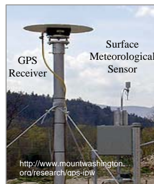
Figure 4: GPS-PWV configuration in Bartlett, NH
