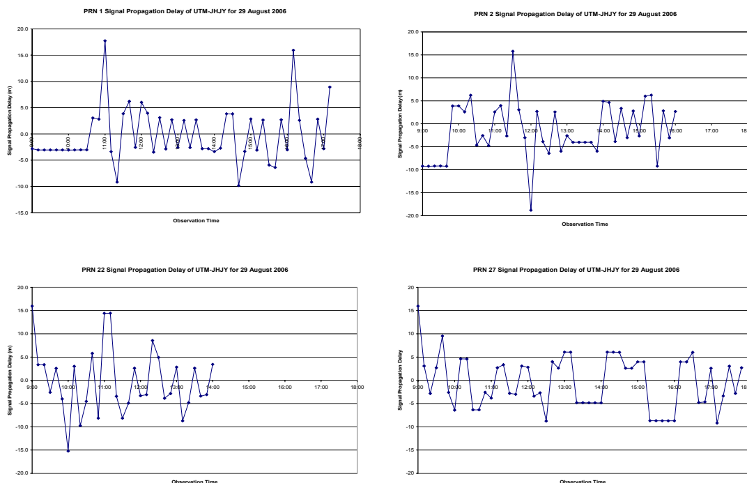
Figure 4.9: Signal Propagation Delay of a) SV 1 b) SV 7, c) SV 22, d) SV 27 in UTM-JHJY Baseline for 29 August 2006
