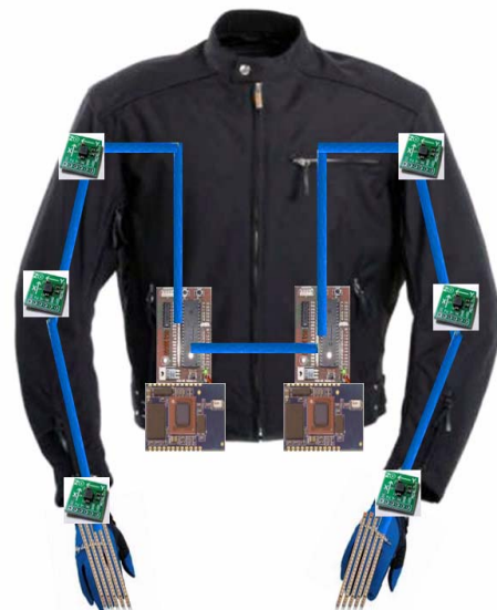
Figure 4: Overall Hardware Setting for Capturing Hand Gesture.
