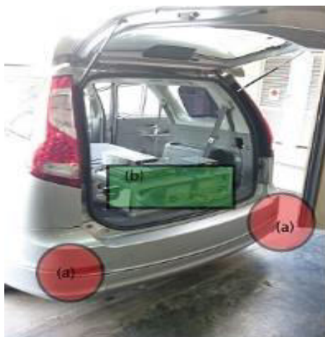
Figure-6. Test Vehicle: (a) blind spot detection radar; (b) MicroAutoBox II.
