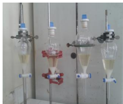
Figure 1. Experimental set up of alcoholysis of Jatropha curcas oil produce two phase materials, which are biodiesel and glycerol
